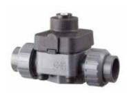
The flow coefficient (C<sub>V</sub>) represents the flow rate in gallons per minute (GPM) at 68°F for which there is a 1 psi pressure drop across the valve in the fully open position. These values are determined from an industry standard testing procedure which uses water as the flowing media (specific gravity of 1.0). To determine specific flow rate and pressure loss scenarios, one can use the following formula:
